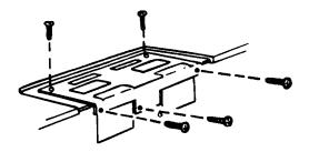
9. Remove 2 screws on front of grille. Remove grille.
